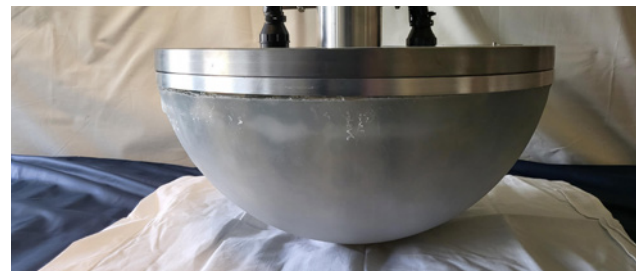
Figure 2a: Hemispherical Indenter, ANSI/RESNA SS-1:2019 section 6. Image for illustration purposes, not actual test rig used.
